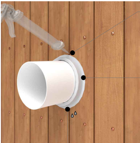
No sealant to drain
