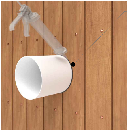
Continuous weather seal around pipe
